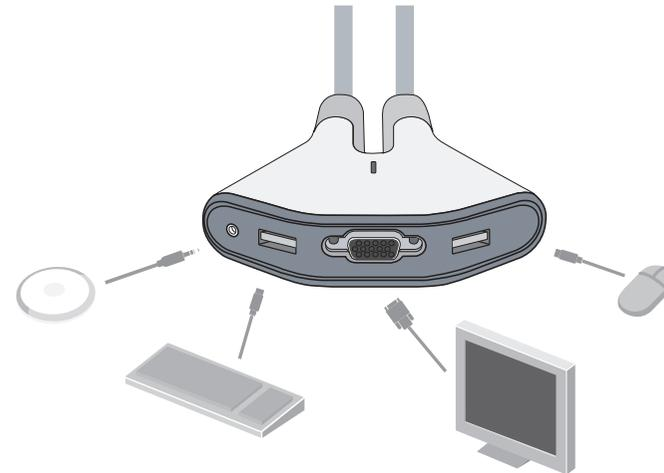
3. Connect one set of cables to the monitor and USB ports on your first computer. Wait for your computer to recognize the new USB device (Flip). Then connect the other set of cables to the monitor and USB ports on your second computer.
