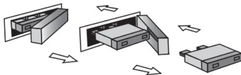
**2. Replace the blown fuse with a new spade type fuse**
