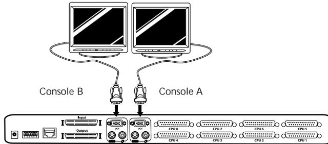
2. Connect the PS/2 keyboard cable to the keyboard port on the back of the MATRIX2 in the "Console A" section.
