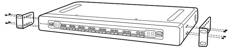
1. Determine how far you would like the MATRIX2 to protrude from the rack. Select a bracket-hole scheme.
