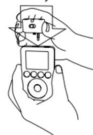
Insert the Microphone Adapter into the iPod's remote connector.
