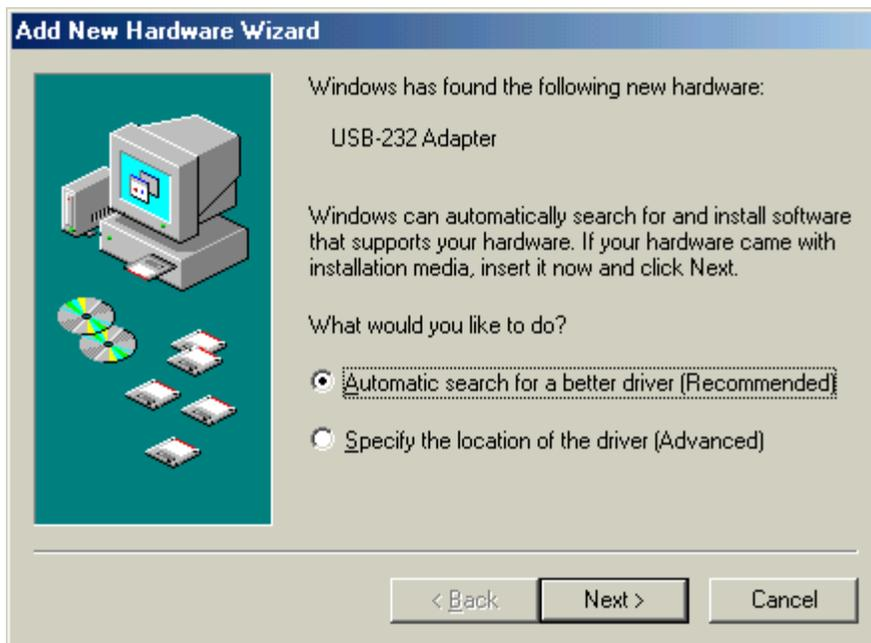
4. Windows will then search for the software. It will find the two files listed below. Select the USB to Serial Converter A:\Serial\Win98\Belu2ser.Inf and click ok.
