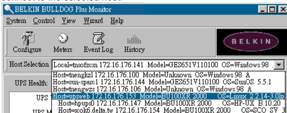
If the host is located on the Internet, you can also input the remote host IP address from the View Menu- Remote Hosts menu shows the hosts you can establish connections with.
