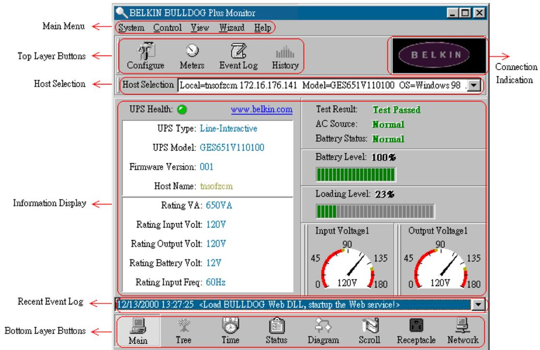
**Host Selection:** Press the combo box to select hosts that runs Bulldog Plus in the LAN. Users can monitor or control the UPS remotely (password is needed).
