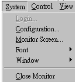
**Login:** Used for Remote Monitor. User must enter the password verification before he can control or configure the UPS.
