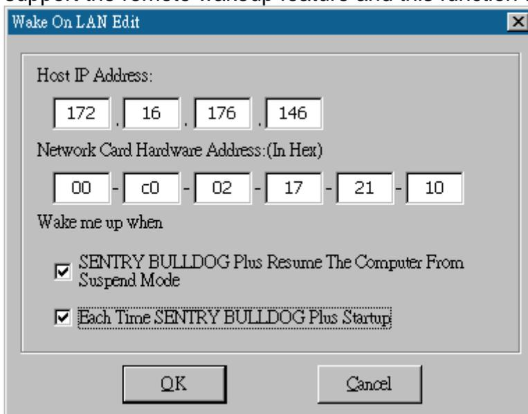
a Bulldog Plus Resume The Computer From Suspend Mode: Bulldog Plus will reinstate the computer into normal mode, and the program will awaken the remote hosts once the actions have been enabled.
