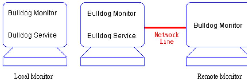
You can run only Bulldog Monitor without running Bulldog Service. Bulldog Monitor will search hosts in the LAN(Local Area Network) which runs Bulldog Service in the combo box. Click on the Host Selection combo box to list the searched hosts in the LAN. Select one, then Bulldog Monitor will connect to the selected host.
