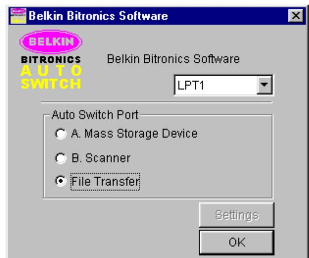
switch act as if it was a file transfer cable. You can now run programs such as Windows® Direct Cable Connection, or Laplink. Please refer to their user manuals or websites for information on how to configure their software. Just remember that your Bitronics switch setup mimics the file transfer cable requirement.
