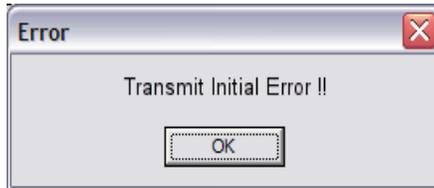
To resolve this click 'OK' and 'OK' again. Unplug Power from the KVM, then unplug the Flash Update Cable. Wait 10 seconds. Now plug the Flash Update Cable in first, followed by the Power Cable (or KVM Cable Kit). Repeat Step 4.
