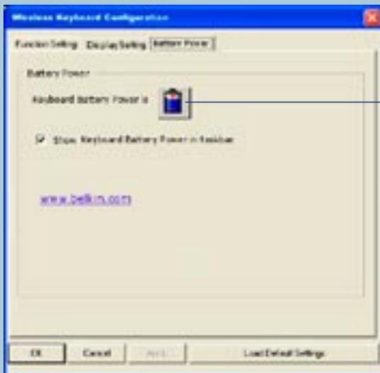
1. "Keyboard Battery Power" shows battery power status.
