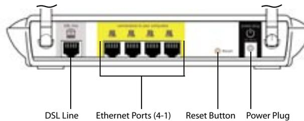
1.3 Connect the telephone cord from the wall jack providing ADSL service to the "DSL Line" port on the rear of the Router.
