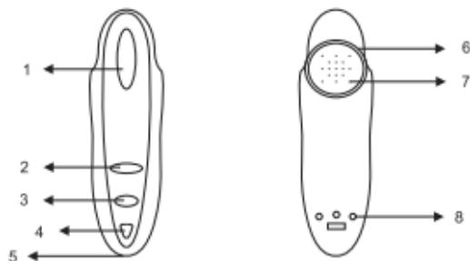
1. **Talk Button:** Switches the headset on/off, answers/ends a call, pairs the headset with a device, and is used for voice dialing.
