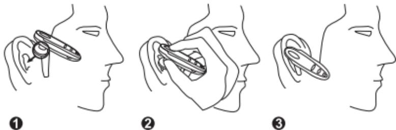
The ear cushion supplied with the Belkin Bluetooth Headset provides additional comfort and Better fitting. To attach the ear cushion,
